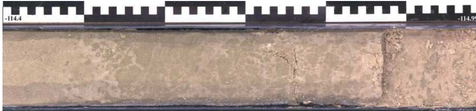
Figure 19. Core section from -114.4 m to -114.99 m; Intense very light green bioturbation of soft very light brown, fine-grained sand between -114.54 m and -114.7 m which then decreases in intensity downwards. Influx of a new sand layer above -114.54 m smothered the biogenic organisms shortly after they had caused some bioturbation of the basal part of the new sand layer (-114.5 m to -114.54 m). In this particular layer, bioturbation only reached to a depth of 45 cm below surface of the sediment, i.e. from -114.54 m to -114.99 m. However, in the core section immediately below this, the bioturbation reaches a depth of 2 m below the surface of the sediment, i.e. from -115 m to -117 m.
