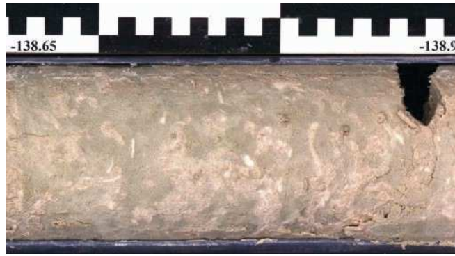
Figure 23. Elongated, thin, white, randomly orientated, calcareous dolocrete nodules which may be rhizoliths; core section -138.65 m to -138.9 m.
