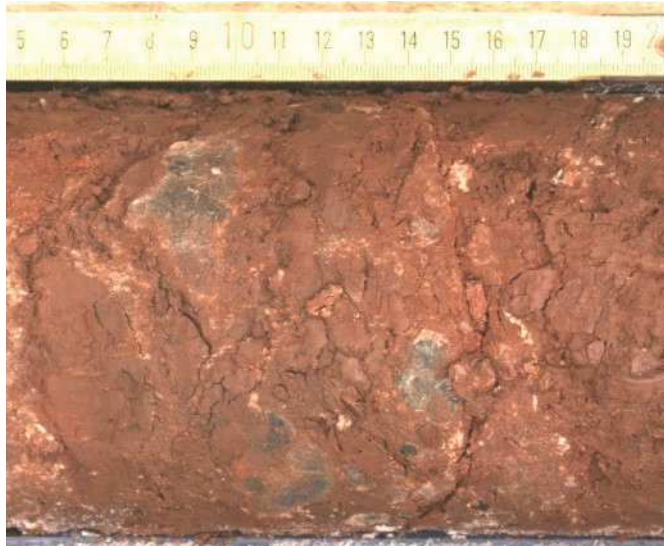
Figure 63. -359.05 m to -359.20 m: Black, knobby calcareous dolocrete and dolomitic calccrete nodules with thin white rims in red clay.
