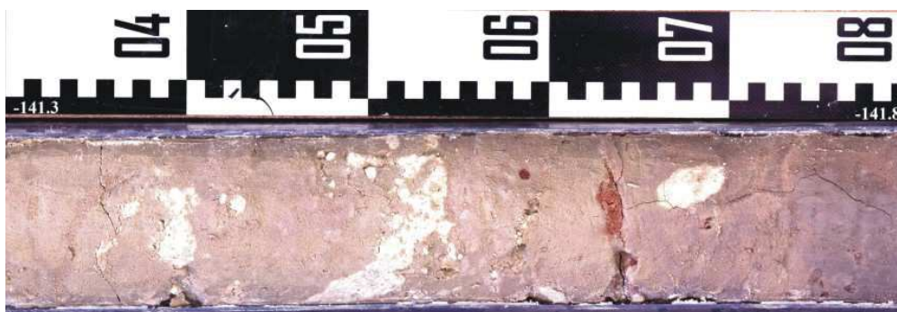
Figure 25. Core section from -141.3 m to -141.8 m. The section from -141.4 m to -141.74 m is a zone of light green sand containing patches of faintly purplish clay. This appears to have been the top of the underlying deep greyish purple clay so intensely bioturbated that there is more light green sand (burrow fillings from overlying sand) than clay. There are two faintly reddish burrows above the mixed zone and two very hematitic burrows in the lower half of the mixed zone.
