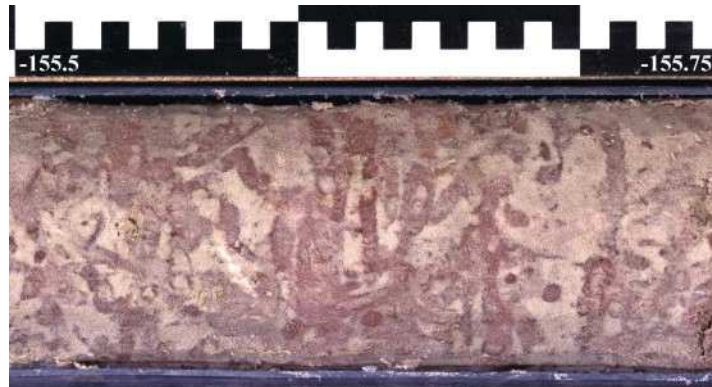
Figure 30. Red, second period burrows with internal, Cruziana -type laminations; core section from -155.5 m to -155.75 m.
