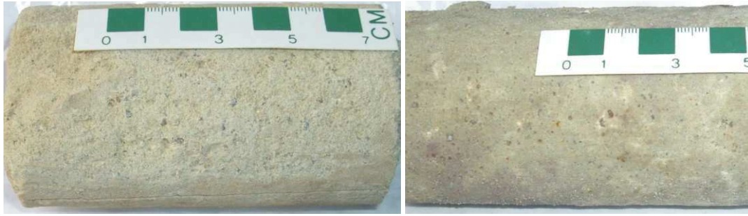
Figure 4. Examples of a few very coarse grains randomly scattered through poorly sorted, clayey, fine- to medium-grained sand in borehole WW 201216: left sample -80.5 m depth; right sample -173.5 m depth; top to the left in each case.
