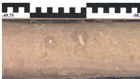
Figure 9.2. Small white calcrete spots. The enclosing sand has been darkened around the spots; core section from -49.75 m to -50.0 m.
