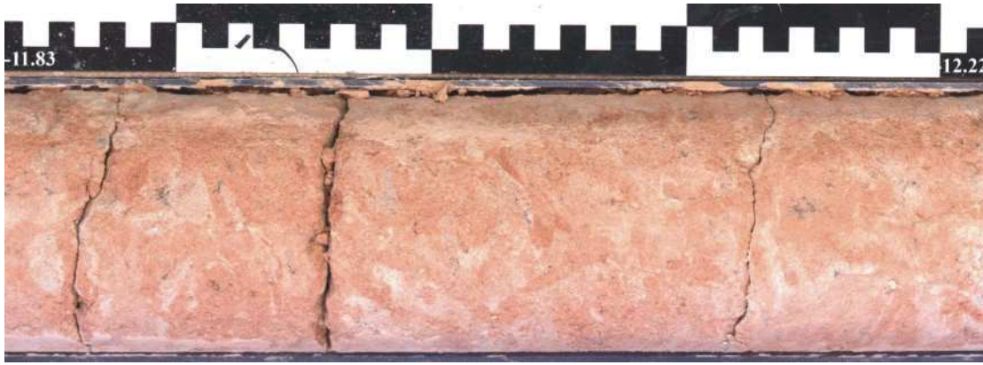
Figure 5. Poorly sorted, calccrete-cemented, fine-grained sand in which the pre-cementation bioturbation burrows/channels are still visible; scale divisions 1 cm; core section from -11.83 m to -12.22 m; top to the left in this and all subsequent figures.
