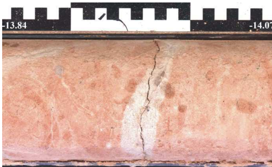
Figure 6. Bioturbation channel with calcified margins and red sand core at -13.9 m in calccrete-cemented, fine-grained sand; bleached calccrete-rich vein; core section from -13.84 m to -14.07 m.
