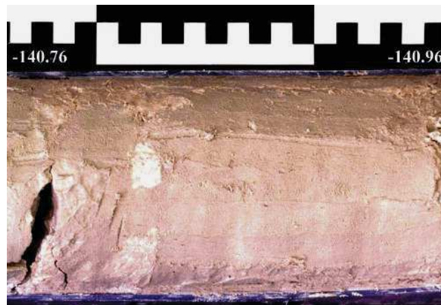
Figure 24. Faint layering (bedding?) forming an angle of about 10° to the core; core section -140.76 m to -140.96 m.
