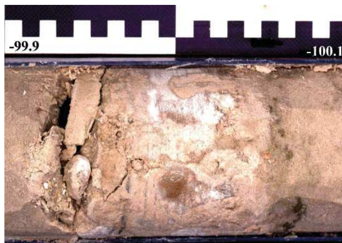
Figure 12. 12 cm thick zone of clustered calcareous dolocrete nodules at -100 m, origin uncertain; core section -99.9 m to -100.1 m.
