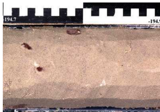
Figure 38. Very light purple patches speckled by numerous tiny dark purple spots (bioturbation?). See also Fig. 41 for similar spots; core section from -196.3 m to -196.7 m.
