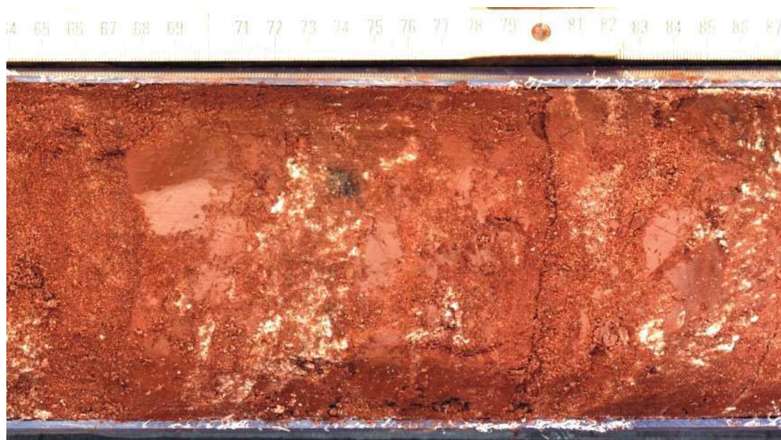
Figure 60. -356.64 m to -356.87 m: Numerous clasts of red clay (paler red) in fine- to medium-grained red sand. Patchy cementing by hard, white calcrete.
