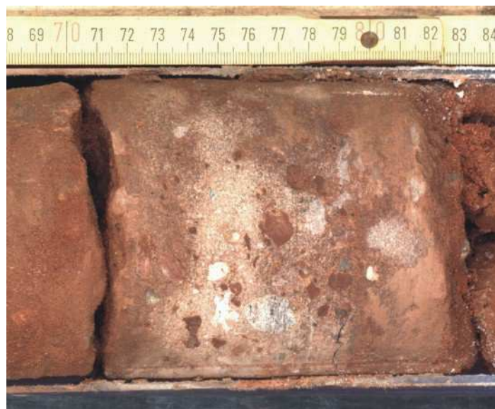
Figure 47. -269.71 m to -269.86 m: Sandy conglomerate layer with intrabasinal clasts of white and grey calcrite and dark red clay. The matrix is cemented by hard white calcareous dolocrete.
