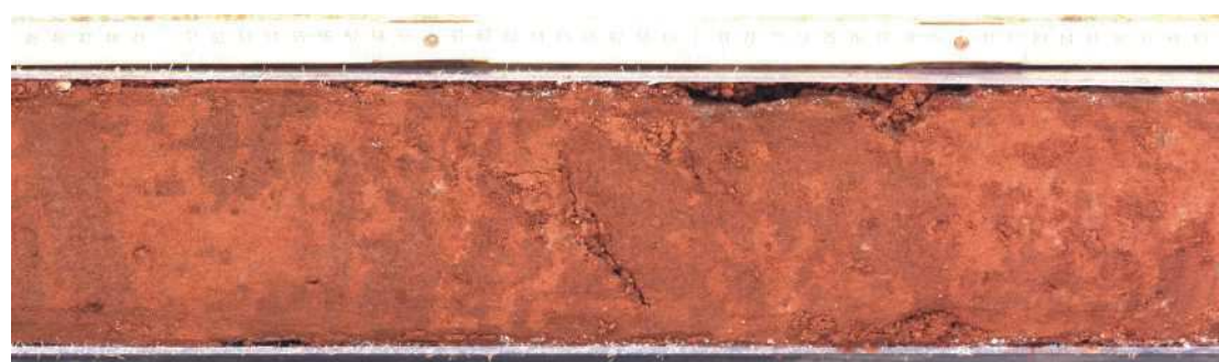
Figure 48. From -273.45 m to -273.90 m is a mixed layer of soft, red, poorly sorted, very silty, very fine-grained sand containing irregular, darker patches of very similar but more clayey sand which may have been mixed during deposition (clasts of one in the other) or by bioturbation.
