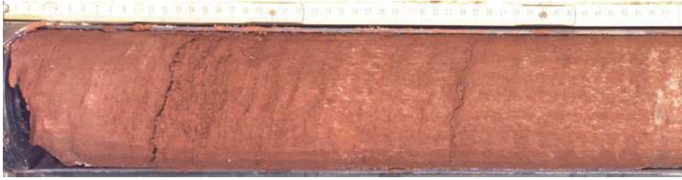
Figure 54. -291.0 m to -291.5 m: Single 42 cm thick cross-bedded unit of red clayey silt from -291.0 m to -291.42 m. The layering forms an angle of about 20° to the core. Horizontal bedding, the norm (cf Fig. 52), in the basal 9 cm of the photograph.
