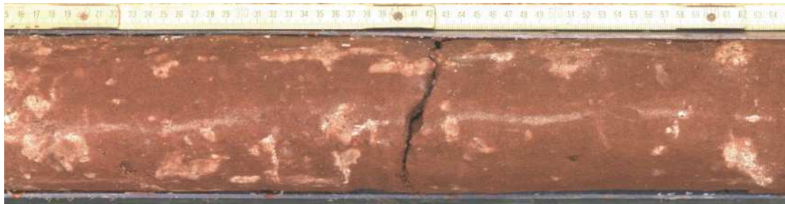
Figure 64. -362.15 m to -362.65 m: An intermittent, 6 mm-wide and 50 cm-long vertical streak that may be a bioturbation channel or burrow.
