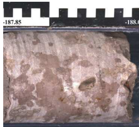
Figure 35. Hard, white, calcareous dolocrete nodule enclosing uncemented, sand-filled bioturbation burrows(?). If these are burrows, they pre-dated the nodule; core section from -187.85 m to -188 m.
