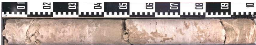
Figure 20. Large, hard calcareous dolocrete nodules, the uppermost one (left) containing round, bioturbation-like burrows filled with sand weakly cemented by calcareous dolocrete. The burrows would have pre-dated the nodule and seem to have escaped the intense cementation of the rest of the nodule; core section from -119 m to -120 m.
