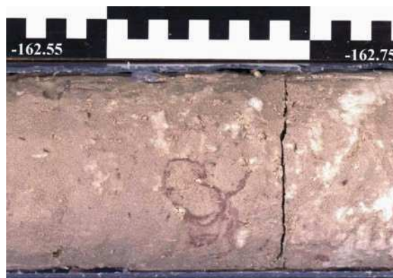
Figure 32. Unusual bioturbation structure with thin red rim and the same coloured sand inside and outside the rim; core section from -162.55 m to -162.75 m.
