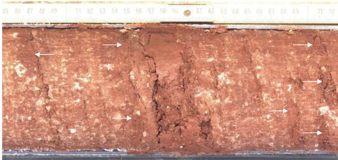
Figure 57. -334.45 m to -334.72 m. Two laminated to very thinly bedded, sandy conglomerate layers with a 2 cm thick clay layer that drapes the top of the lower conglomerate and separates the two conglomerates from each other. Both conglomerates contain small white calcrete clasts and red clay clasts, the larger of which are arrowed.
