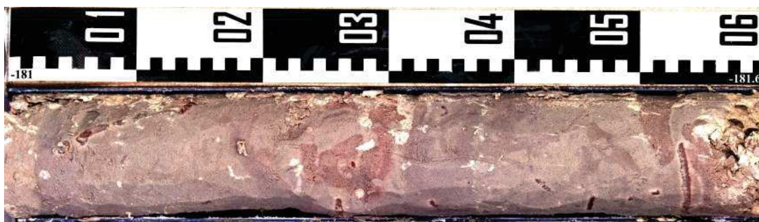
Figure 34. Core section from -181 m to -181.6 m, top of Ohangwena II Aquifer: There is a sharp sedimentary boundary at -181.04 m and a very light grey or purple tinge to the core below that. After the first very light purple and light red bioturbation, the sand was broken up into different sharp-edged coloured patches. Burrowing bioturbation then continued (see long, thin, vertical, slightly sinuous burrow or root channel between -181.3 m and -181.4 m). The dark red burrows seem to be the youngest, note the bleaching of the sand around them and the Cruziana -type lamination in the burrow at -181.54 m (diagenetic reduction of organic matter?).
