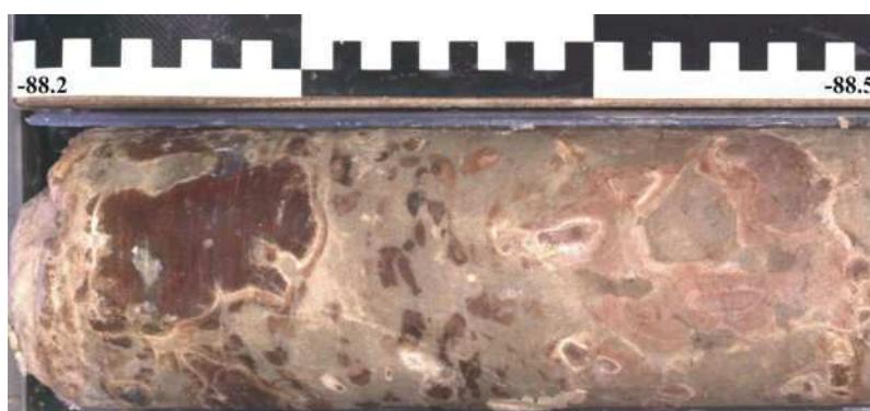
Figure 11. Dark red silcrete and light pink dolocrete nodules set in a hard, very light green matrix of fine-grained, clayey sand cemented by dolocrete; core section from -88.2 m to -88.5 m.
