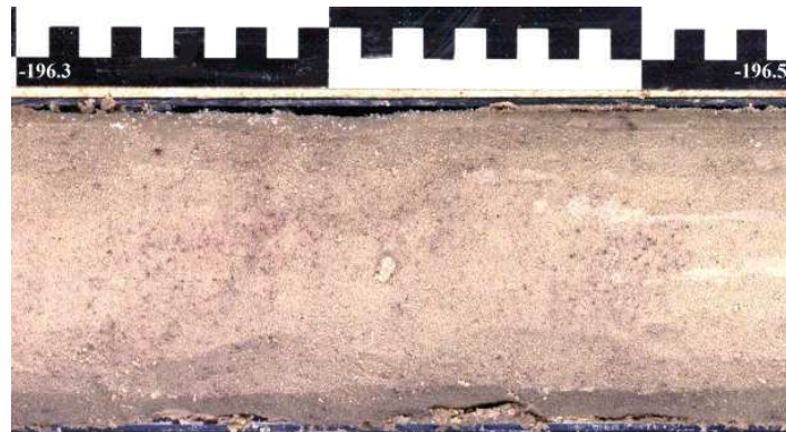
Figure 38. Very light purple patches speckled by numerous tiny dark purple spots (bioturbation?). See also Fig. 41 for similar spots; core section from -196.3 m to -196.7 m.
