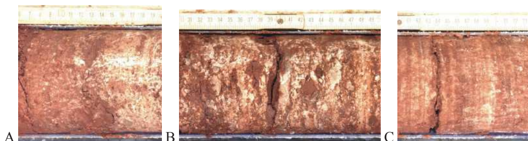
Figure 55. Sandy conglomerate layer containing intrabasinal clasts. The matrix sand is cemented by calcareous dolocrete. A: -325.06 m to -325.2 m; upper part, a few small clasts of white calccrete, large red clay clasts. B: -325.3 m to -325.5 m; thinly bedded middle part, many white, a few grey calccrete clasts up to 2 cm in diameter, red clay clasts up to 4 cm long, latter flattened in the bedding. C: -325.6 m to -325.74 m; basal laminated part with a few small white calccrete and red clay clasts.
