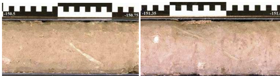
Figure 27. Left: Calcified rhyzolith; core section -150.5 m to -150.75 m. Right: Faint light purple bioturbation burrows; off-white, long, less calcified rhyzolith; core section -151.35 m to -151.6 m.
