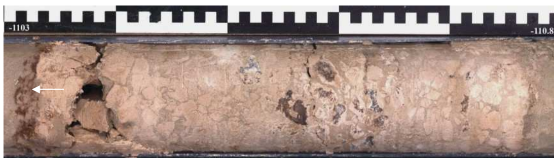
Figure 14. The third of the four, stacked, nodular pedogenic calcareous dolocrete layers. The matrix between the nodules is a very light green, poorly sorted, fine- to very fine-grained, highly silty sand cemented by calcareous dolocrete; note (i) the irregularly shaped cores of dark brown silcrete in the dolocrete nodules in the middle part of the section, the silcrete being a replacement of the dolocrete, (ii) the thin disrupted layer of dark brown clay on top of the dolocrete (arrowed), and (iii) the very light green sand below the dolocrete; core section -110.3 m to -110.8 m.
