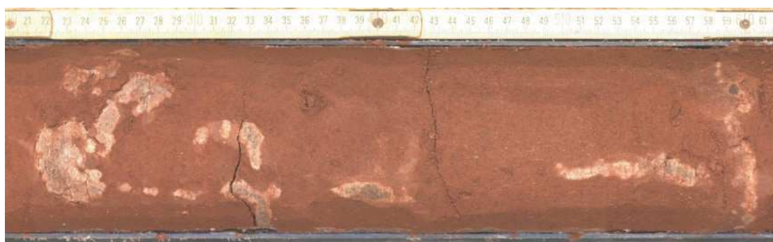
Figure 62. -361.2 m to -361.62 m: Unusual elongate, calcareous dolocrete nodules parallel and perpendicular (rhizoliths?) to bedding in red, consolidated, slightly clayey silt; note zoning of nodules - grey cores, white rims.
