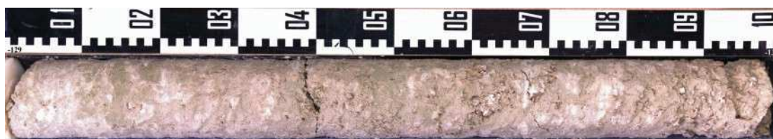
Figure 22. Soft, light green, very clayey, poorly sorted, fine-grained sand choked by smallish, hard dolocrete and calcareous dolocrete nodules; core section -129 m to -130 m.
