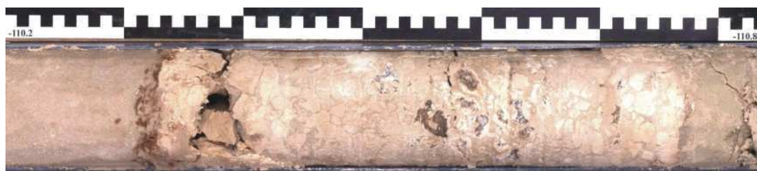
Figure 15. Same section as Fig. 14 but showing more of the sands above and below the dolocrete. The sand below is very light green, the colour probably being due to very intense bioturbation of an originally very light brown sand (see later). The same very light green sand forms the matrix to the dolocrete fragments indicating that the dolocrete formed within the very light green sand, very likely just below the surface of the sand. The subsequent depositional episode probably washed away the cover of green sand above the dolocrete and deposited a very light greyish yellow sand (very light brown in the photograph) which was not subsequently bioturbated. This suggests either (i) a long break in sedimentation allowing the dolocrete to form, and/or (ii) a significant change in depositional conditions between deposition of the lower very light green layer and the upper very light yellow layer, (iii) or preferential carbonate deposition along the contact between the two differently coloured layers where the dark brown clay layer occurs; core section from -110.2 m to -110.84 m.
