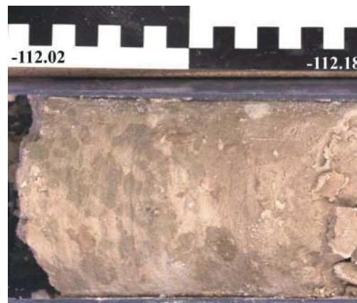
Figure 17. The lowermost 12 cm of the pedogenic dolocrete of Fig. 16. This contains fewer nodules and more of the very light green matrix sand and is typical of basal parts of pedogenic calcretes. The sand in the lower 8 cm of the figure is very light brown, soft, fine-grained and clearly different in colour from the matrix sand of the dolocrete; core section from -112.02 m to -112.18 m.
