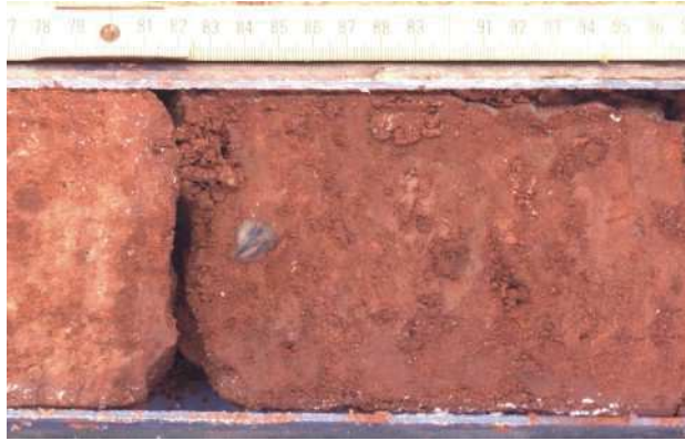
Figure 49. Grey chert nodule at -276.84 m in red, soft, very silty, very clayey, poorly sorted, very fine-grained sand. Sand above the nodule cemented by hard white calcrete.
