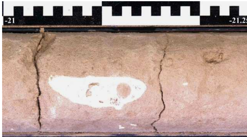
Figure 7. White calcrite nodule in poorly sorted, fine- to medium-grained sand weakly cemented by dolocrete, faint bioturbation burrows to the right of the nodule; core section from -21 m to -21.25 m.
