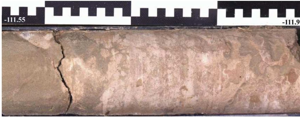
Figure 16. The second of the four stacked, nodular pedogenic calcareous dolocrete layers. It occurs below very light green (intensely bioturbated?), poorly sorted clayey sand. There are fewer nodules in the lower 15 cm of the dolocrete. The soft matrix of the dolocrete is of the same very light green, clayey sand. Thus, the pedogenic dolocrete formed within the very light green clayey sand; core section -111.55 m to -111.9 m. Fig. 17 occurs immediately below this dolocrete.
