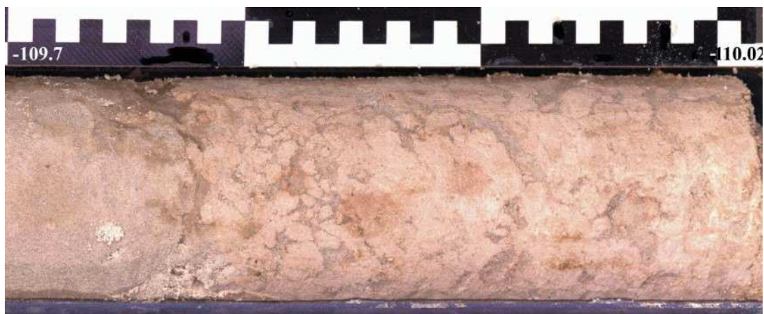
Figure 13. Clustered nodules of a 23 cm thick pedogenic calcrete, uppermost of the four stacked pedogenic calcrete/dolocrete layers; core section -109.7 m to -110.02 m.
