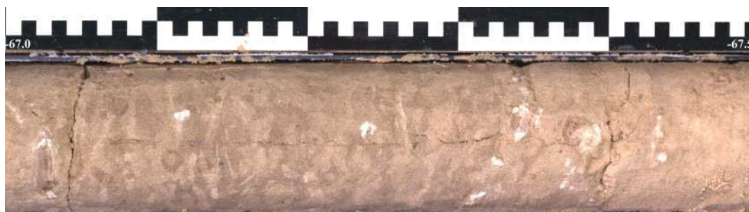
Figure 10. Distinct bioturbation of hard, fine-grained, moderately well-sorted, dolocrete-cemented sand, note zoning of some of the bioturbation channels; core section -67 m to -67.5 m.
