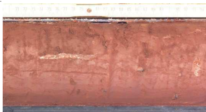
Figure 53. -290.7 m to -290.95 m: Long, vertical, rhyzolith-like calcrete nodule in red clay.
