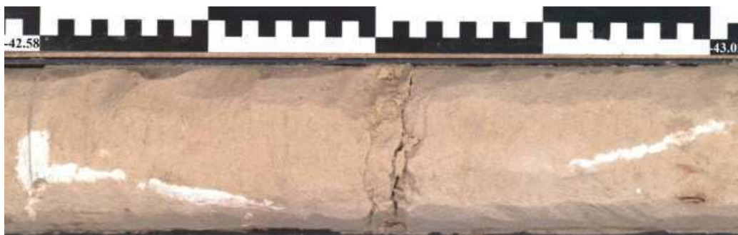
Figure 9.1. Possible calcified rhyzoliths in soft, fine-grained, moderately well-sorted sand of the Ohangwena I Aquifer; core section from -42.58 m to -43.02 m.
