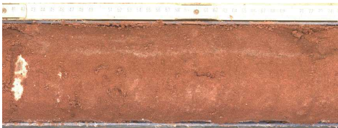
Figure 69. -372.4 m to -372.75 m: Faint, white, vertical bioturbation channel or burrow.
